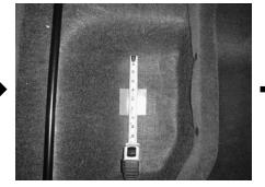
**STEP 2:** Remove the paper backing and place supplied wax square onto the floor.
