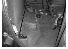
**STEP I:** Remove the passenger side metal floor extension, if so equipped.
